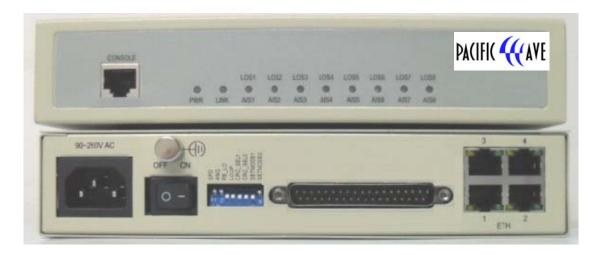
PW-4E1-4ETH is the IP over TDM converter, which supports the conversion from MAC frames to  $1\sim4$  E1 lines. The maximum bit rate is 7.936Mbps (4E1 lines). The device shows estate and alarm information of each E1 channel, and also offers a RS232 port, which is used to connect NMS server which has been installed GUI NMS software. Compliant to international standards, the device can communicate with products from other manufacturers adopting the same standards.
